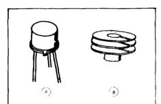
fig. 1. (*A*) Typical low-signal (low-heat transistor) does not use a heatsink. (*B*) Top-hat finned heatsink helps power transistors run cooler.
